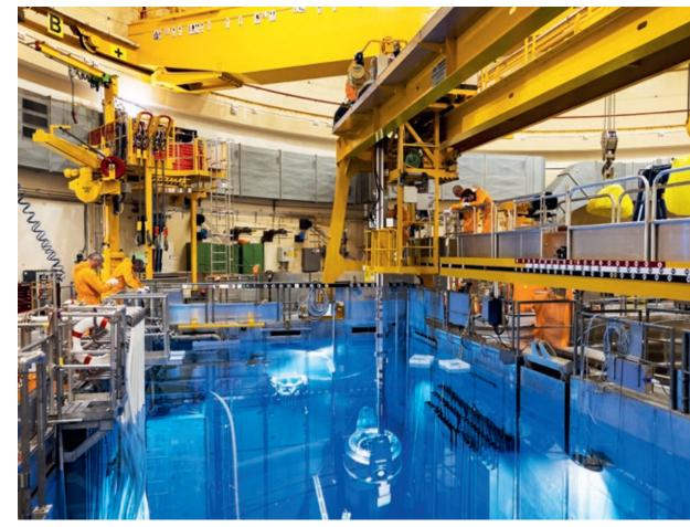
loaded under water into the special container with which they are transported to the interim storage facility.
